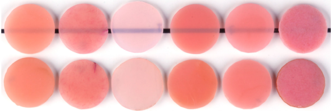
FIGURE 3 Representative specimens demonstrating translucency against a black line (top row) and color change following staining (bottom row). Materials are (left to right): Ivotion Base Milled Denture Base, Lucitone 199, Dentca Denture Base II, High Impact Denture Base, Lucitone Digital Print 3D Denture Base, TrueDent Resin.
